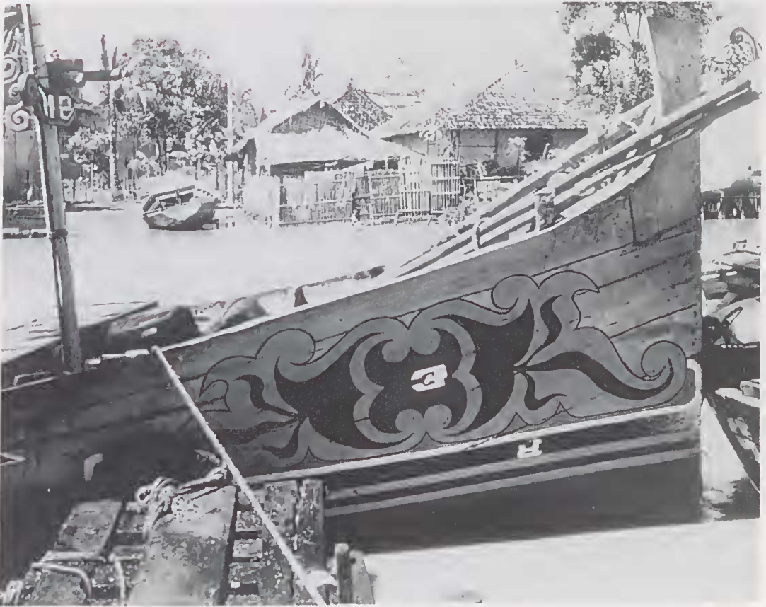
Fig. 31. The bow of a Javanese jegongan showing the lack of a stem, the plank pattern and the prow finial.
